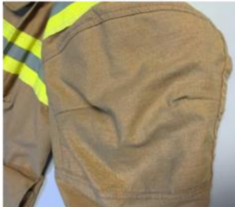
Competitive Design 4 seam elbow design
